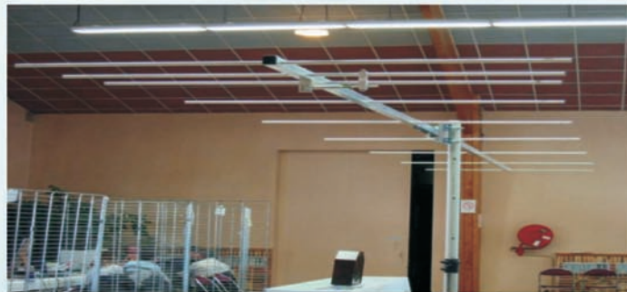
DX.S.R 902 Boom 25x2mm 30x2mm elements 10x1mm
