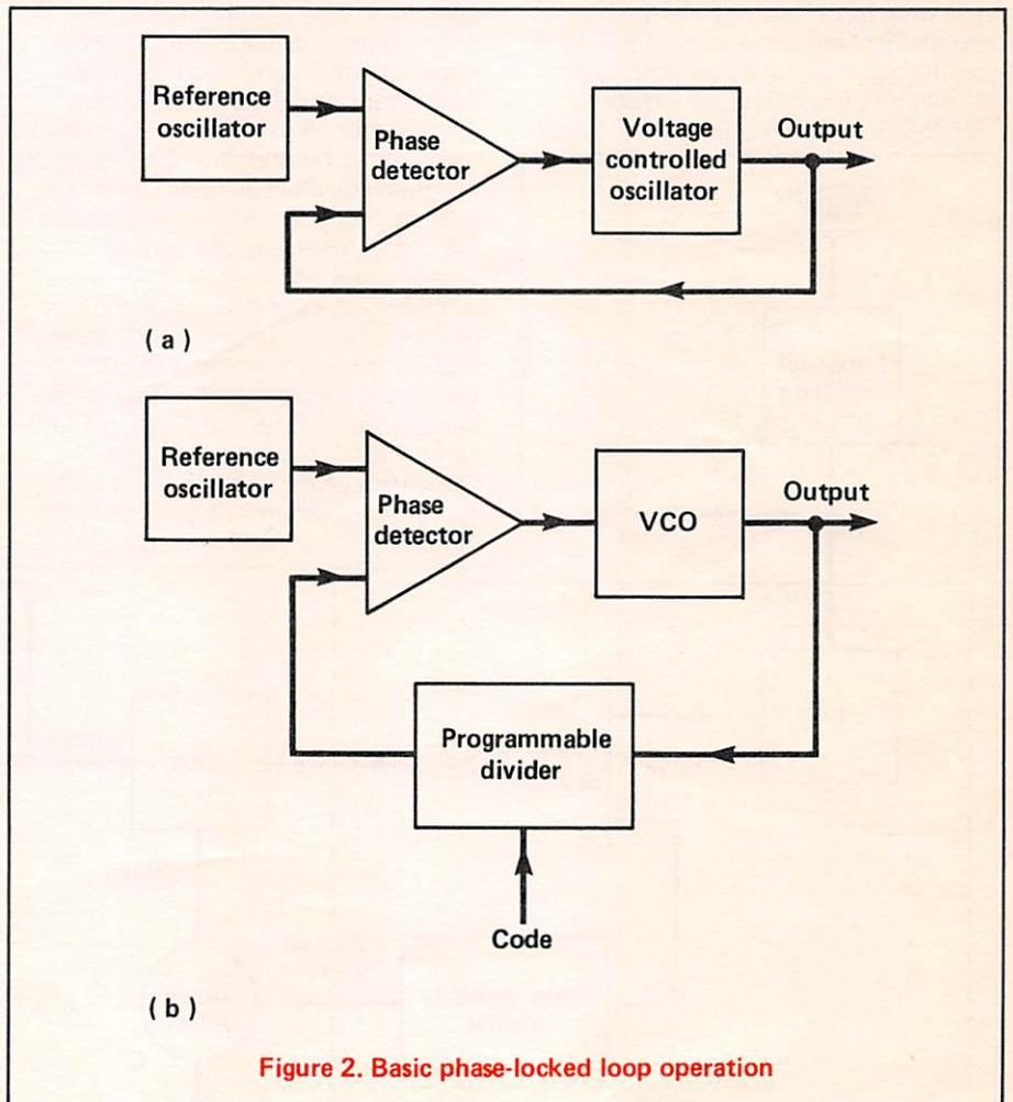
Figure 2. Basic phase-locked loop operation
