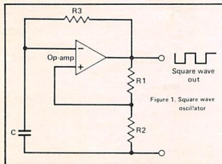
op-amp, via the resistor R3 and into the capacitor. When the voltage at the (-) terminal of the op-amp exceeds that at the (+) terminal, the output switches to low, or negative. Now, the capacitor discharges and when the voltage at the (-) terminal becomes lower than that present at the (+) terminal, the output switches to high again. The cycle simply repeats over and over to produce the output tone.
