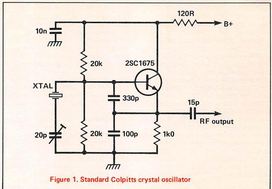
Figure 1. Standard Colpitts crystal oscillator
