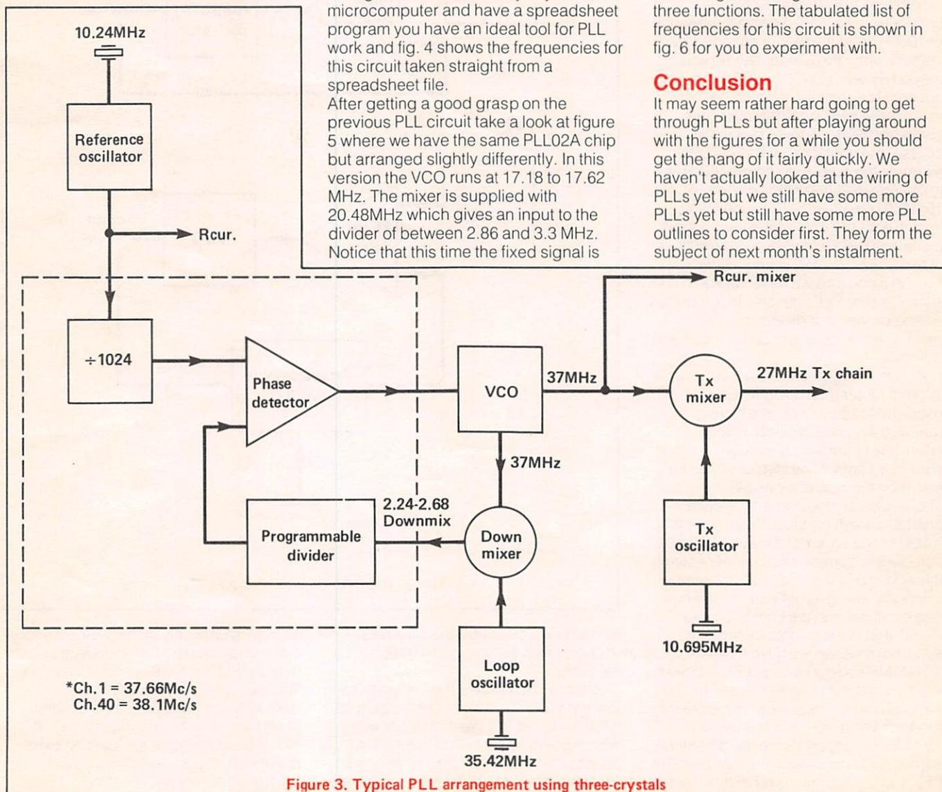
Figure 3. Typical PLL arrangement using three-crystals
