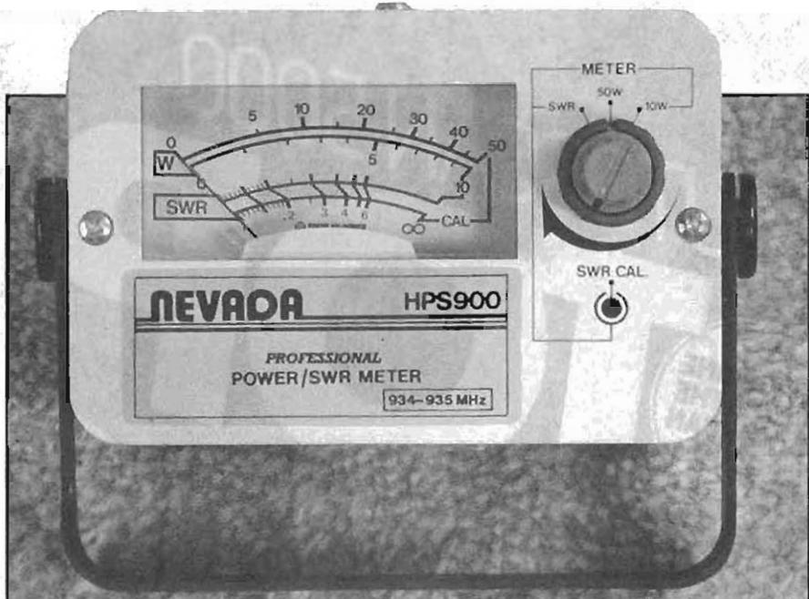
The Nevada SWR meter from Telecomms. It has been designed for the UK market and also measures power.
