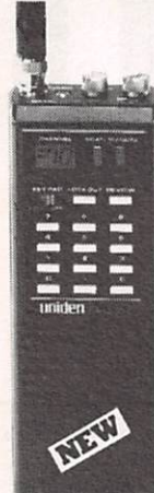
MODEL BC 50 XL Handheld scanning receiver with 10 memories. Covers: 66-88Mhz, 136-174Mhz, 406-512Mhz £99.99
