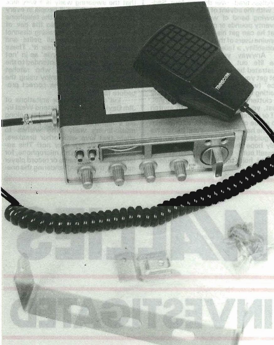
The Transcom GBX 4000 complete with fixing kit.
