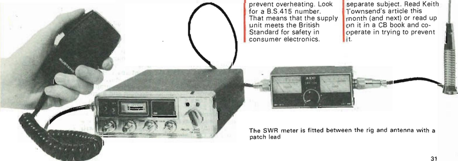
The SWR meter is fitted between the rig and antenna with a patch lead
