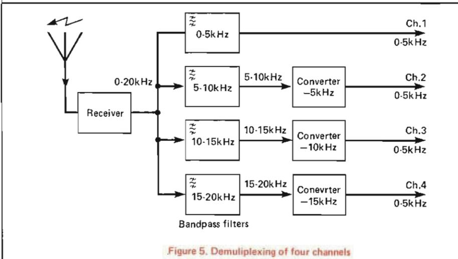
Figure 5. Demultiplexing of four channels
