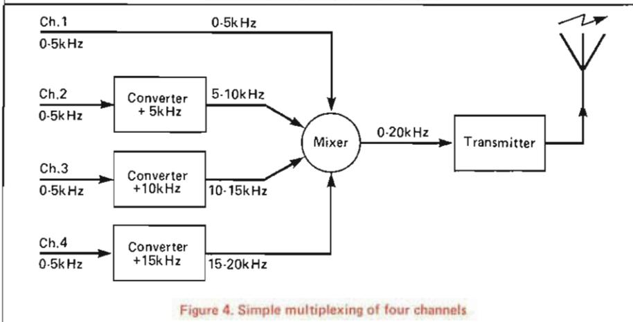
Figure 4. Simple multiplexing of four channels
