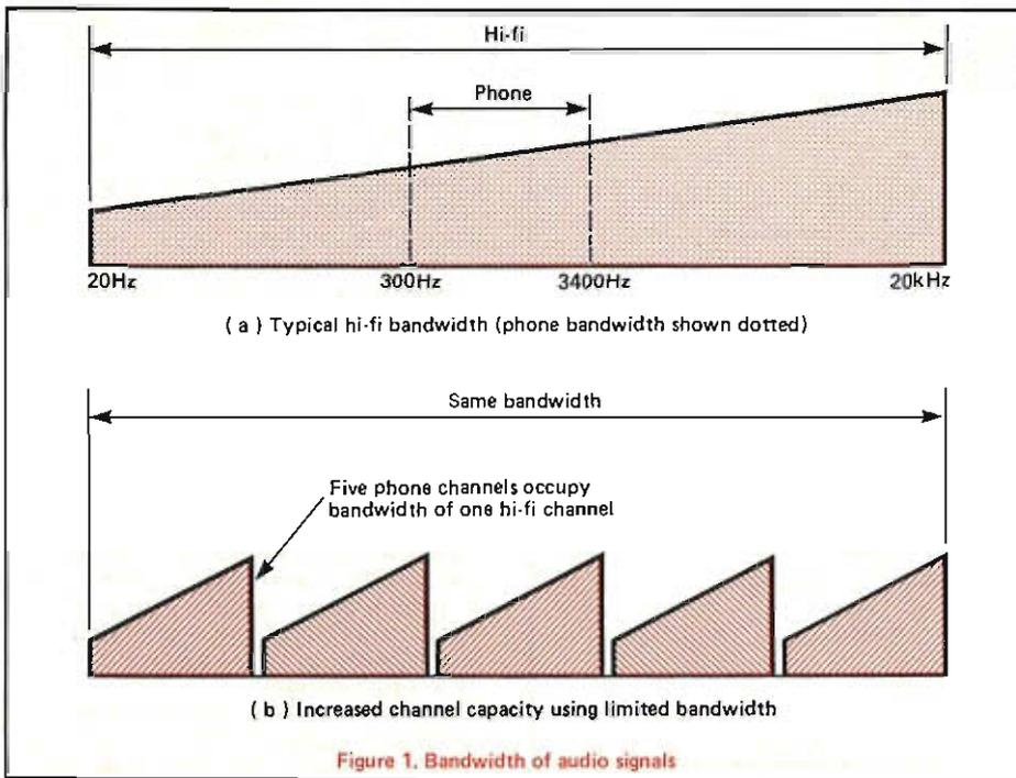
Figure 1. Bandwidth of audio signals
