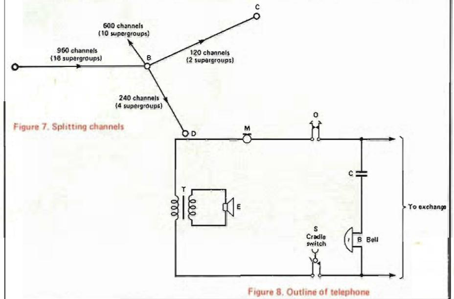
Figure 7. Splitting channels
