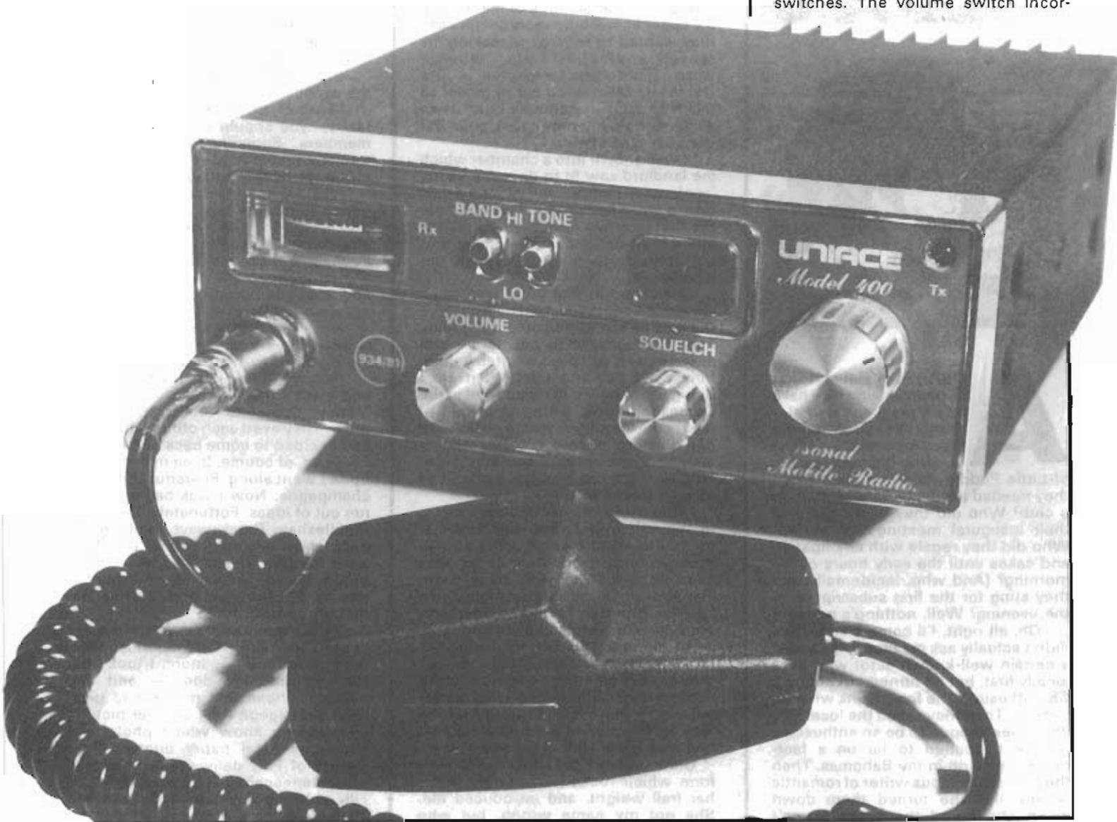
porates an on/off switch as one might expect. The squelch control also has a click position at one end, however. This selects a pre-set squelch level that should be correct for most circumstances.
