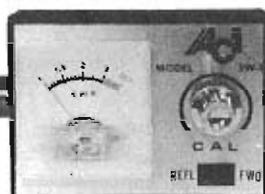
The SW-1 SWR meter measures only 75 x 55 x 45 mm which makes it ideal for mounting permanently under your dashboard because it takes up so little room. It is a single meter device which means that the REFL - FWD switch on the front of the unit has to be used when setting it up. Also on the gold front of the box is a golden CALIBRATE knob. There are two SO 239 sockets on either side of the box.
