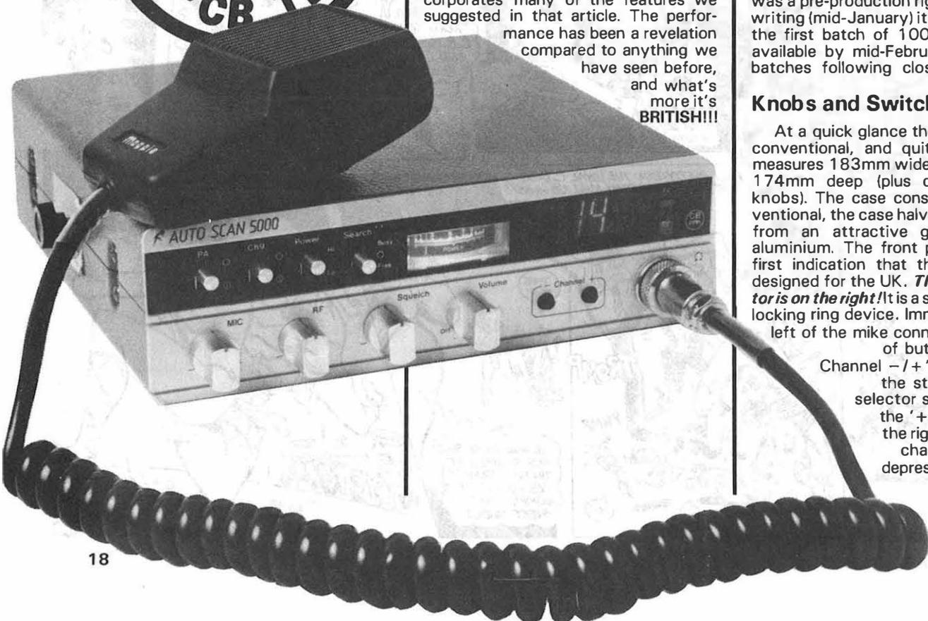
to count up through all the channels. At channel 40 the counter resets to 01 and then continues. The '-' works in a similar manner, counting down. An ingenious touch is that pressing BOTH buttons automatically selects channel 14. Both buttons are repeated on the microphone, for easy operation whilst driving. Continuing from right to left across the lower front panel are four knobs for Volume/off, squelch, RF gain and mike gain.
